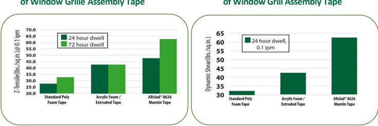
Z-Tensile Strength of Window Grille Assembly Tape
